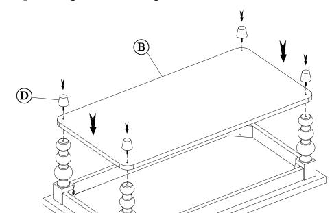
Step 3: Using the Allen key tighten all leg bolts, then hand tighten the bun feet.
